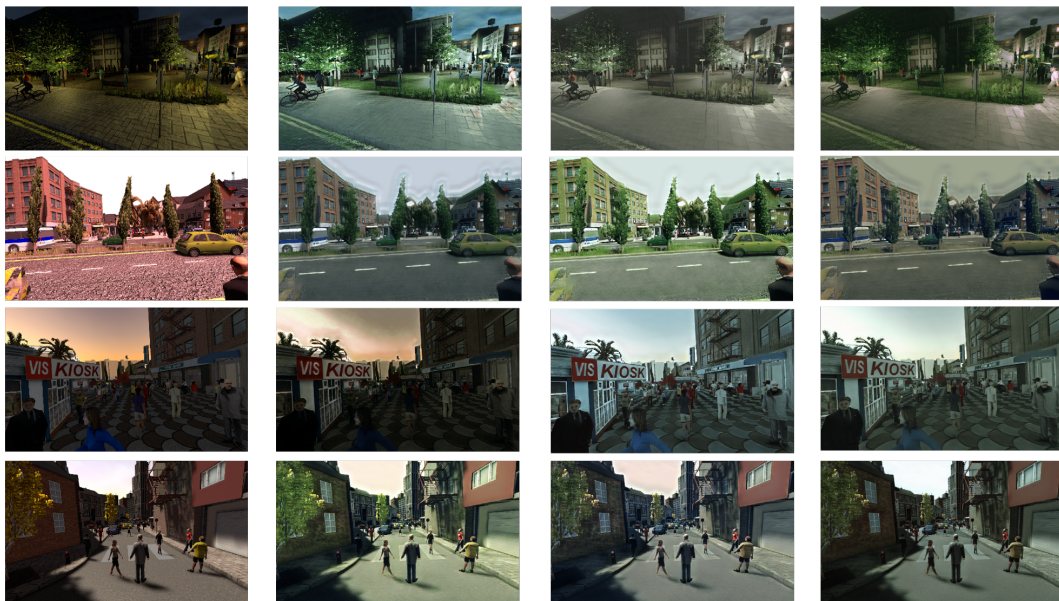
Figure 6.5: Diverse translations of images from the SYNTHIA source dataset to the Cityscapes target dataset: we observe that even though the content and pixel semantics stay intact, we generate diverse variants of the same scene, effectively capturing more faithfully the data distribution in the target domain.
